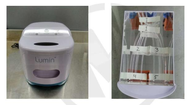
Note: The numbers in the right hand picture indicate the approximate position of the carriers during testing.
